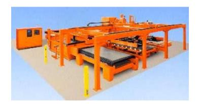
In 1998, Metcam added laser cutting capabilities to its arsenal of fabrication equipment. This first system has a 3,000 watt laser, integrated into a material handling system. The material handling system includes a six shelf material storage tower and automated load/unload. The system is capable of handling two lasers without modification.
